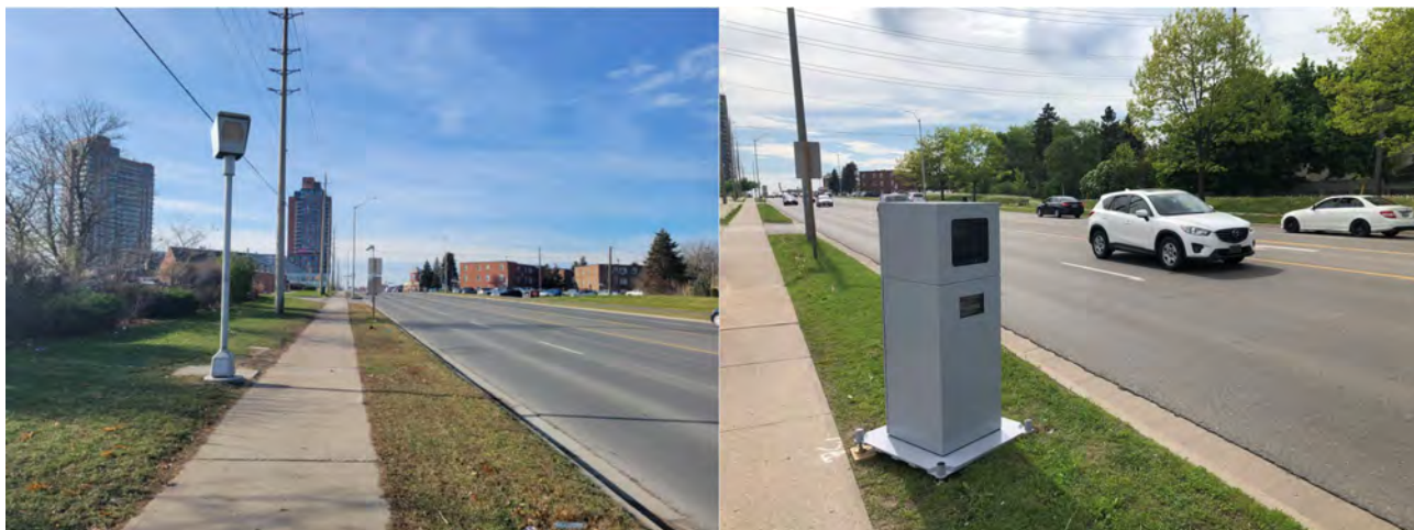
Figure 4 - Permanent (left) and Mobile (right) A.S.E. Cameras
