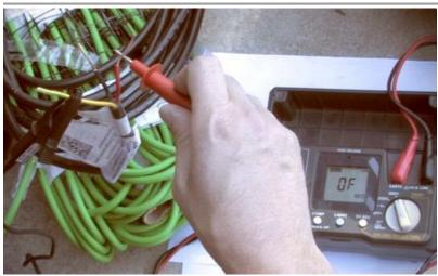
Testing your snow melting system with an ohmmeter and megohmmeter at every stage of installation will allow you to be certain that the heating element is functioning properly.
