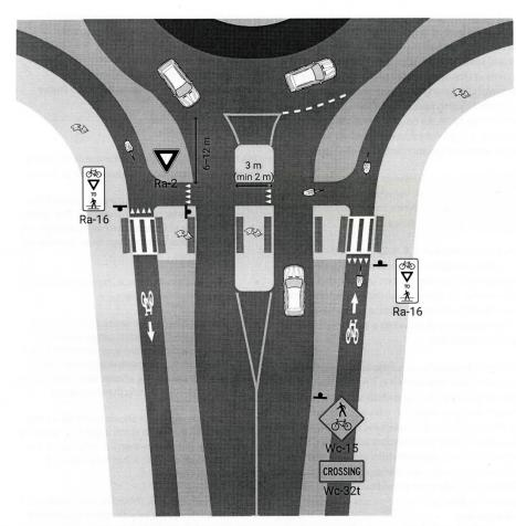
Figure 6.80 - Single-Lane Roundabout, Uncontrolled Crossing Treatment (Motorist-Priority)
